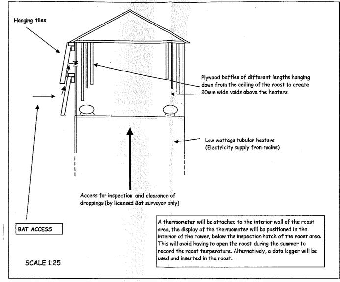
The plywood baffles hanging from the interior of the roosting compartment will ensure that a range of conditions are created. As the tubular heaters heat the air, the air temperature within the 20mm wide void between each baffle will vary dependent on the distance from the heater.
